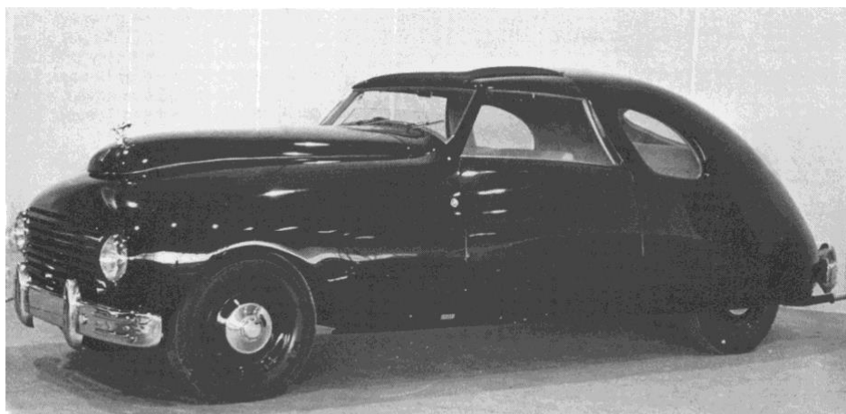
Rolls-Royce Silver Wraith, Chassis-Number #LWAB63 Chassis only exhibited on Rolls-Royce' stand at 1948 Earls Court Motor Show, London. Delivered to France where Poberejski of Paris built this streamlined Sedanca de Ville with revolutionary front design that showed only the mascot of the traditional radiator - and in this form the car was exhibited at 1949 Geneva Show. Rumour has it that Rolls-Royce insisted on this car to be taken away from the show area within 24 hours and the manufacturer refused to issue a guarantee. That might be the reason why the same year a 2nd body was fitted by Franay of Paris - a Drophead Coupé to an elegant though rather conservative design.
